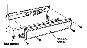
Replace the access panel and toe panel. The toe panel must be positioned to contact floor.
